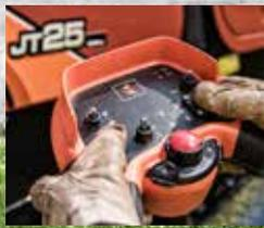
6 Optional wireless remote ground drive increases flexibility when moving the rig and allows fine-tuning of bore path placement.
